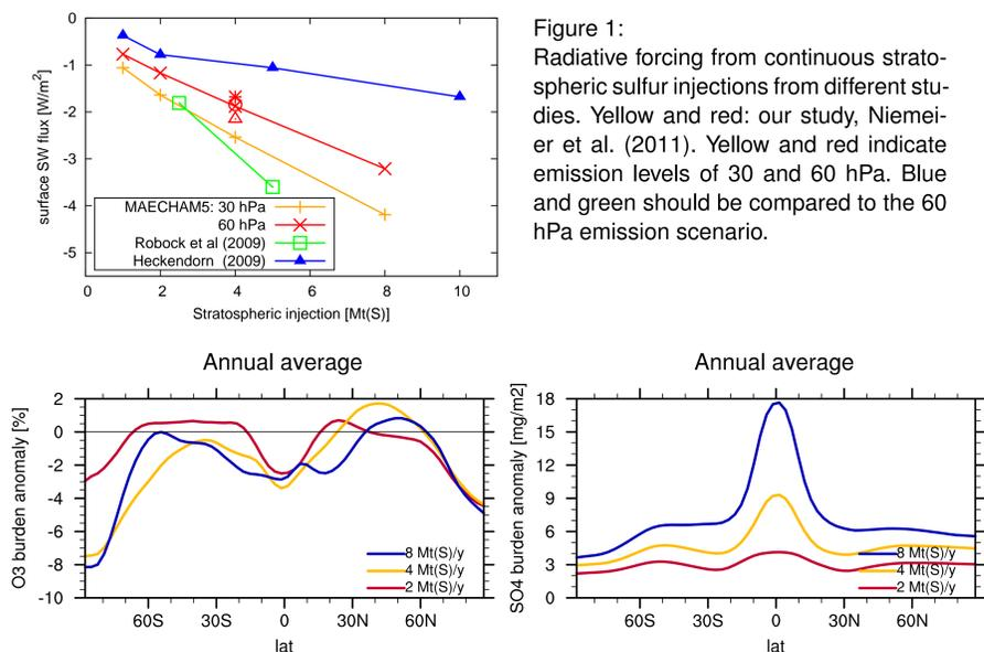
Figure 1: Radiative forcing from continuous stratospheric sulfur injections from different studies. Yellow and red: our study, Niemeier et al. (2011). Yellow and red indicate emission levels of 30 and 60 hPa. Blue and green should be compared to the 60 hPa emission scenario.
