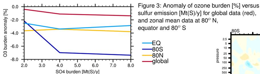
Figure 3: Anomaly of ozone burden [%] versus sulfur emission [Mt(S)/y] for global data (red), and zonal mean data at 80° N, equator and 80° S
